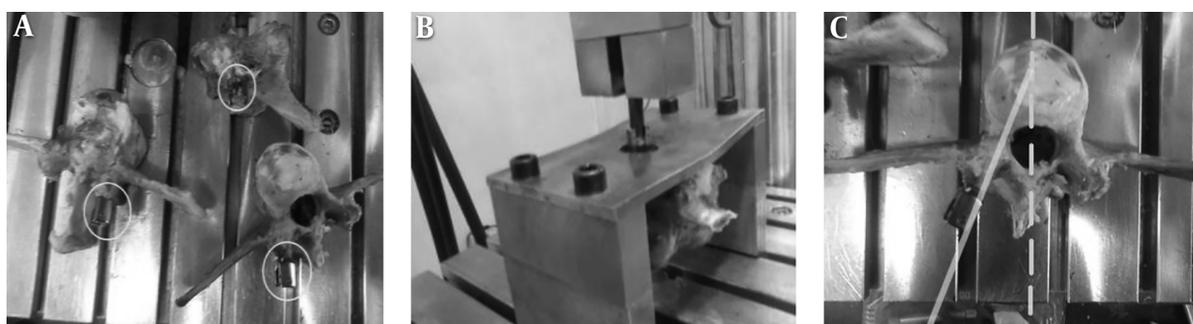
**Figure 2.** A, Preparing bovine lumbar vertebrae and inserting screws into pedicles; B, Bovine vertebra with a pedicle screw mounted in tensile machine; C, The insertion angle of pedicle screw relative to the sagittal line
